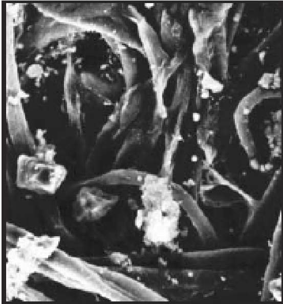
Cellulose filter media with ISO Fine Test dust loading (left). Nanofiber filter media with ISO Fine Test Dust loading (right)
