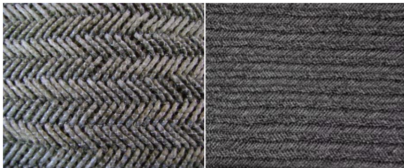
Figure 21 Examples of braided cloth. Left hand side from 22% carbon fiber co-mingled tows, right hand side from 13% carbon fiber co-mingled tows. The bottom axis of both images is equal to 100mm.
