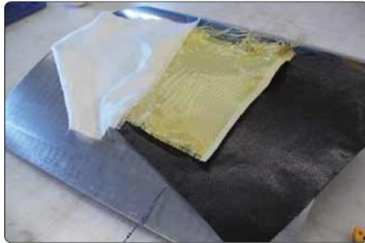
Figure 16 Fiberglass (left), Kevlar (middle), and carbon fiber material (right) [27].
