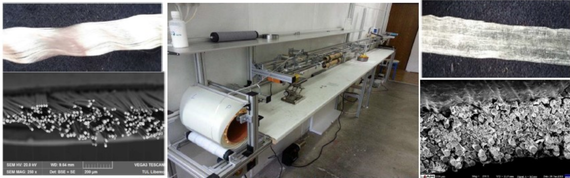
Fig. 10 Prototype line for production of hybrid tapes
