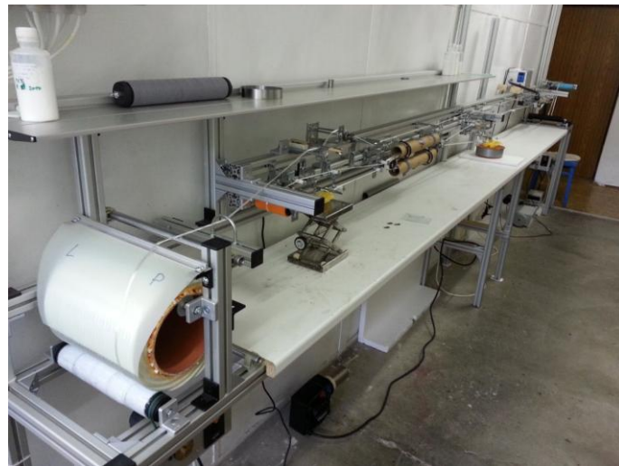
Fig 2. Semi-operating device for preparing a prepreg
