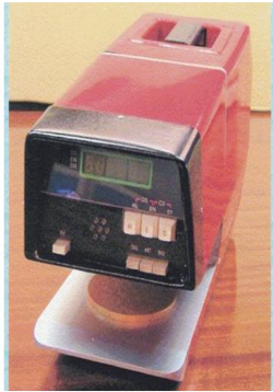
Computer-controlled instrument ALAMBETA for fast measurement of thermal insulation and thermal-contact properties of compressible materials like textile fabrics
