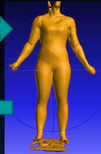
Combined individual scans in a global coordinate system with irregularities
