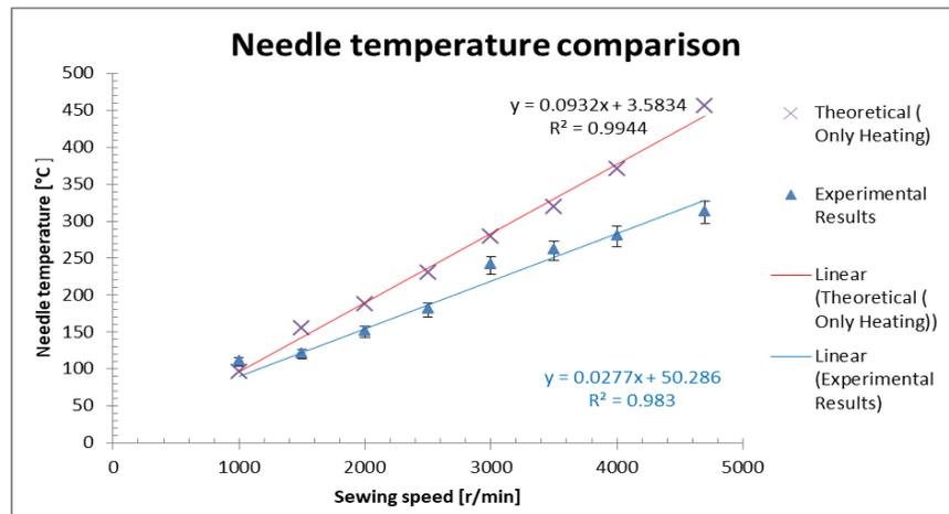
Figure 5. Comparison of experimental and theoretical results.
