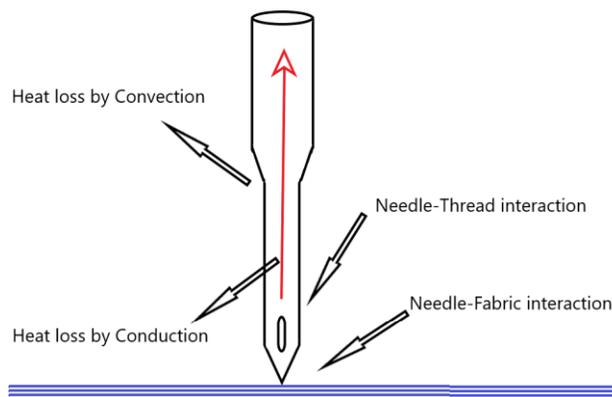
Figure 2 Needle heat balance
