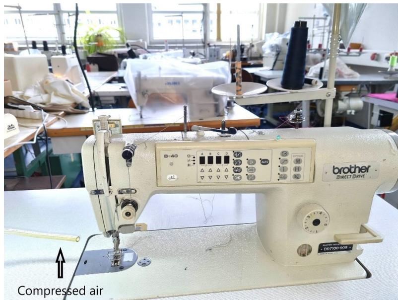
Figure 31 compressed air cooling for hot needle
