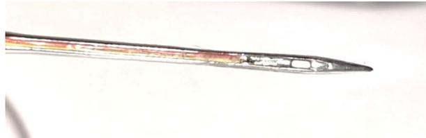
Figure 12 K type thermocouple embedded in needle
