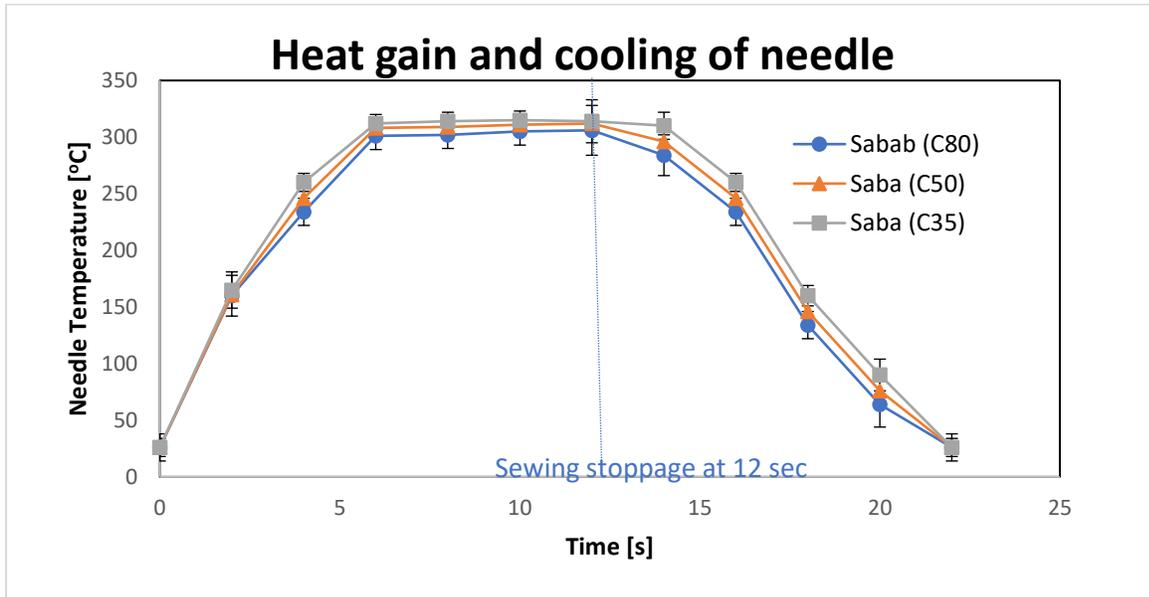
Figure 16 Needle heat gain and loss
