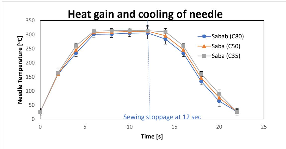
Figure 16 Needle heat gain and loss
