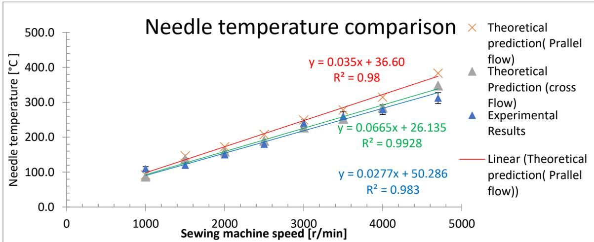
Figure 28 Theoretical and Experimental needle temperature comparison
