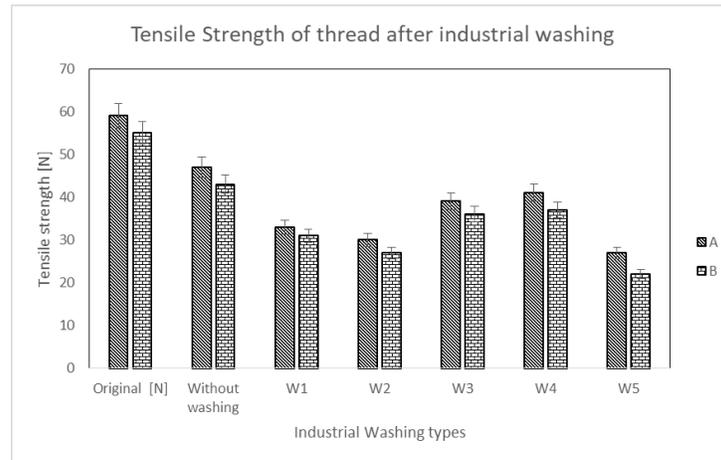
Figure 41 Effect of washing on the tensile strength
