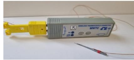
Figure 11 wireless device connected with needle
