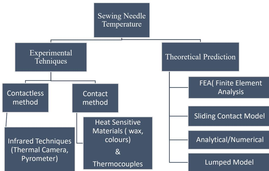
Figure 8 categories of the temperature measurement of sewing needle
