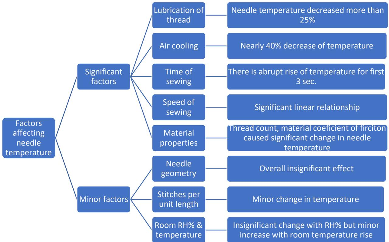
Figure 18 Effect of factors on needle temperature
