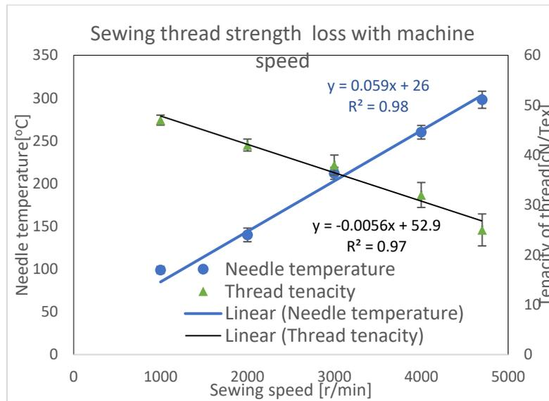
Figure 39 Needle temperature, machine speed and strength of sewing thread
