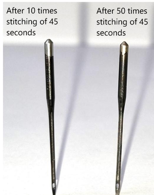
Figure 30 DLC needle after usage
