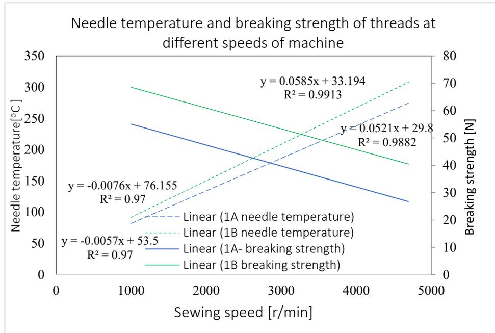
Figure 40 Needle heating and breaking strength of threads
