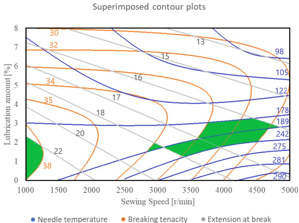
Figure 37 Contour plot of PET-COTTON to show impact of lubricant amount
