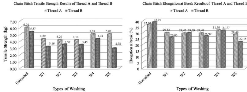
**Figure 6.** Chainstitch tensile strength and elongation at break results of Thread A and Thread B.
