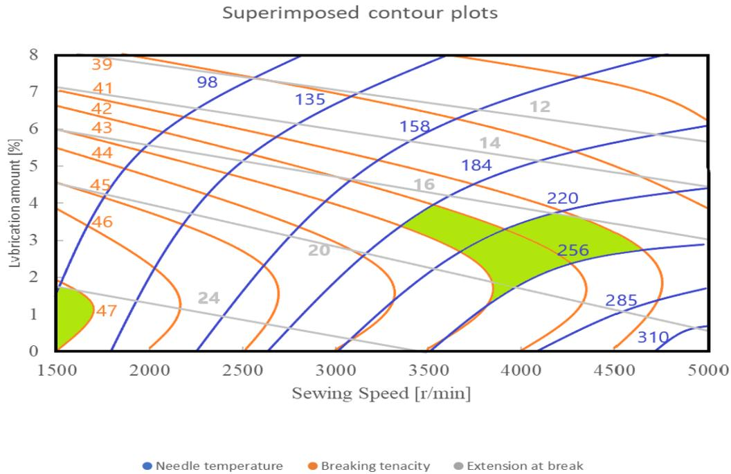
Figure 36 Contour plot of PET core spun thread showing effect of lubricant amount
