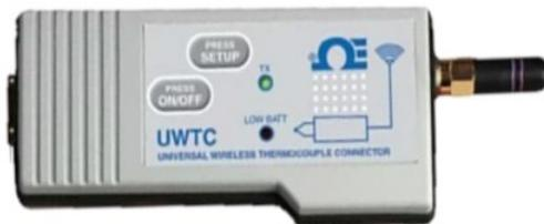
Figure 13 Wireless device UWTC for quick response
