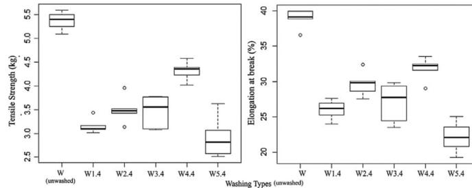
**Figure 4.** Box plot for thread B's chain stitch tensile strength and elongation at break.
