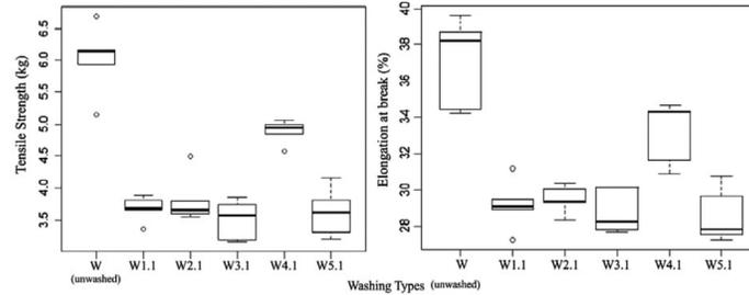
Figure 1. Box plot for thread A's lockstitch tensile strength and elongation at break.
