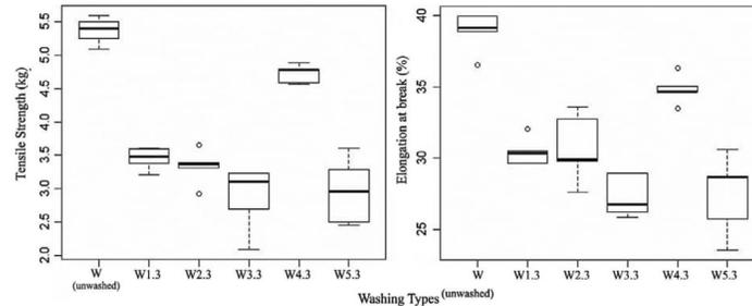
**Figure 3.** Box plot for thread B's lockstitch tensile strength and elongation at break.
