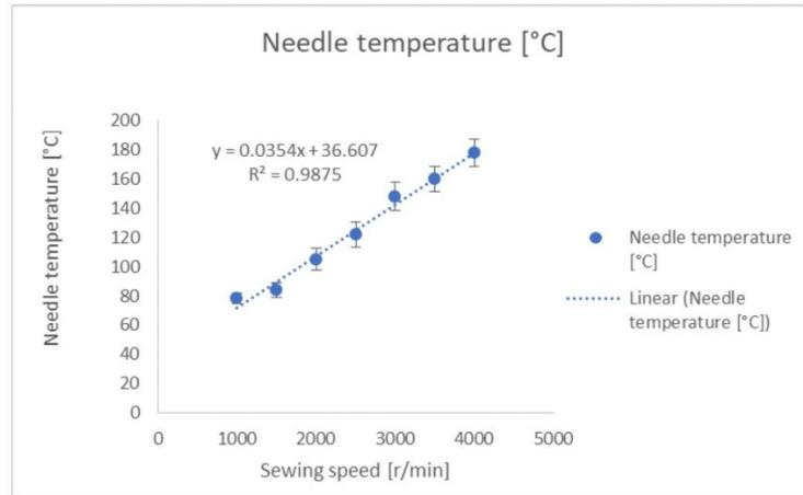
Figure 3. Sewing needle temperature at different sewing speeds.
