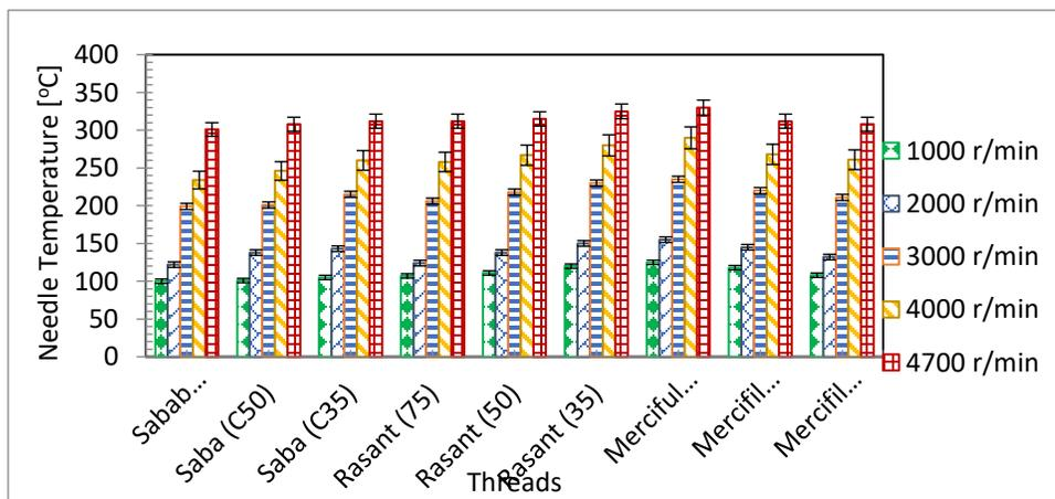
Figure 15 Needle heating with different sewing threads and speed of sewing machine
