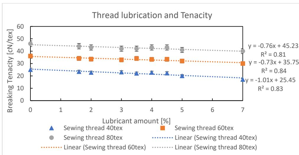
Figure 35 Thread lubrication impact on tenacity
