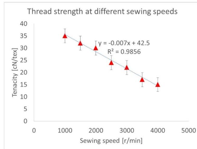
Figure 4. Tensile strength of thread at different sewing speeds.
