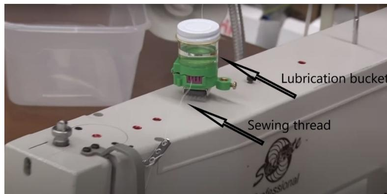
Figure 7 Lubrication setup from company Sailrite®
