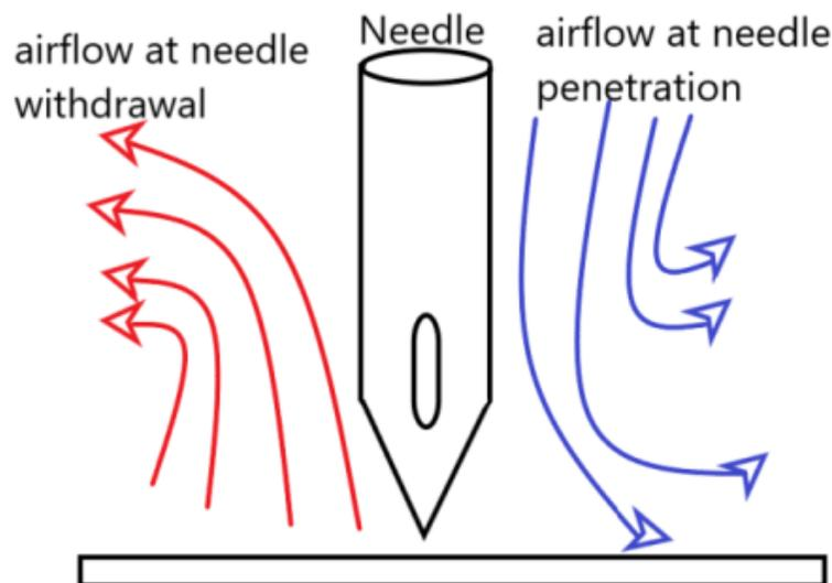
Figure 22 Heat loss by convection with needle penetration and withdrawal
