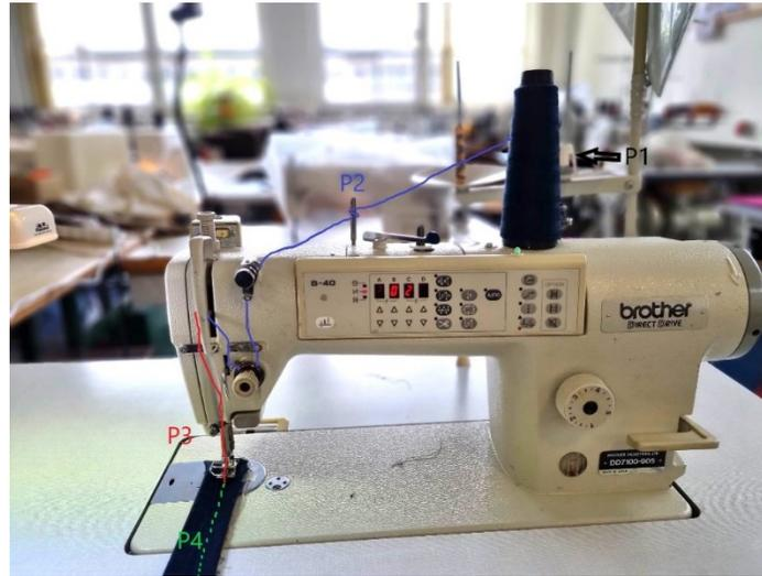
Figure 38 Sections of sewing thread damage
