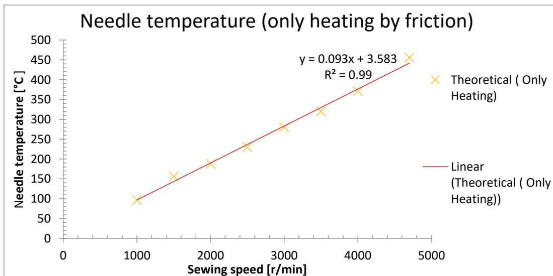
Figure 21 Theoretical prediction of maximum needle heating
