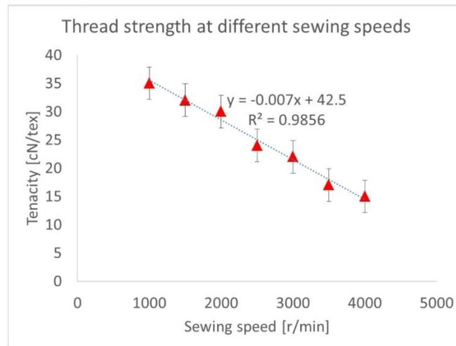
Figure 4. Tensile strength of thread at different sewing speeds.
