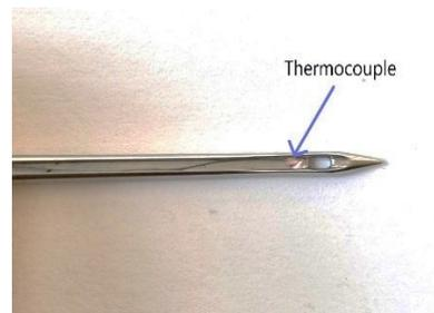
Figure 14 C type thermocouple embedded in needle
