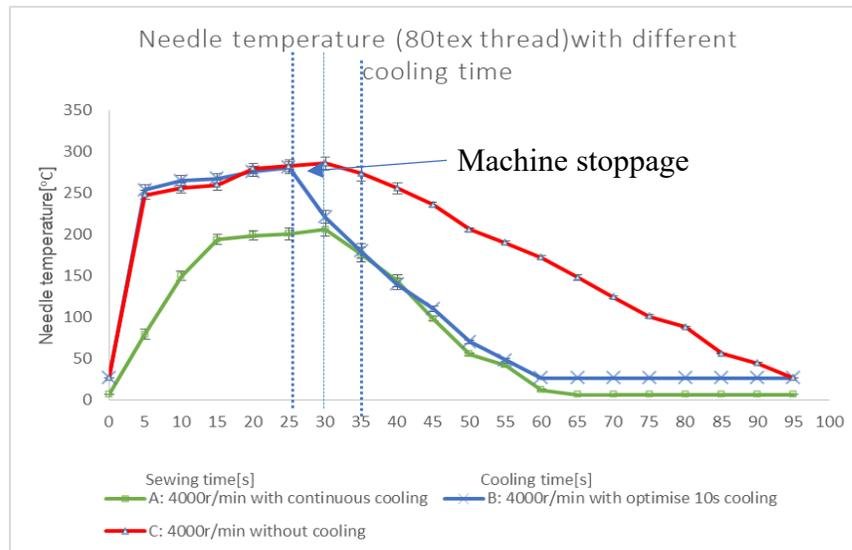
Figure 32 Cooling time and needle temperature
