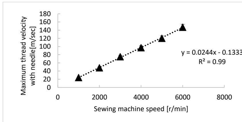
Figure 20 Sewing thread speed
