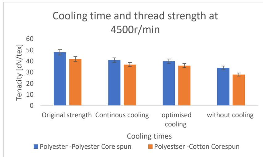
Figure 33 Cooling time impact on the tensile strength of the thread
