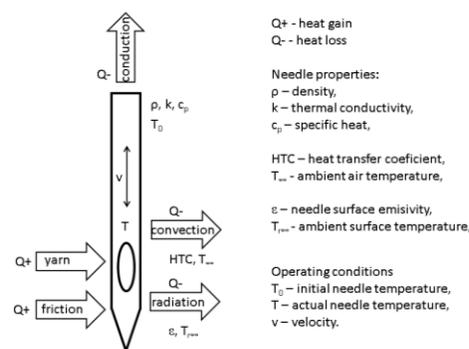
Figure 19 Heat balance of stitch cycle- modified from ref. [26]
