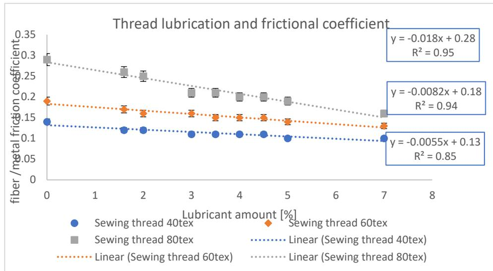
Figure 34 Thread lubrication impact on reduction of frictional coefficient
