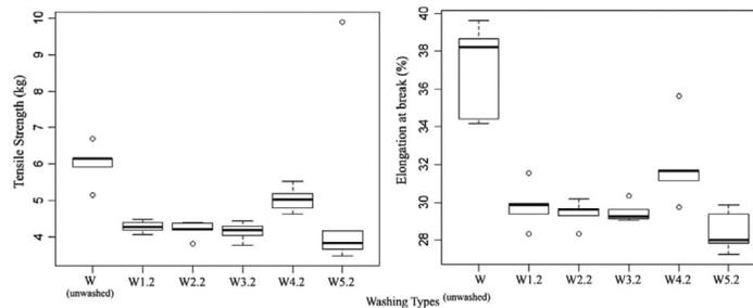
Figure 2. Box plot for thread A's chain stitch tensile strength and elongation at break.
