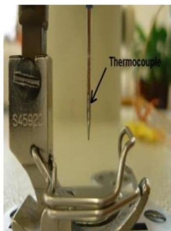
**Figure 2.** Thermocouple embedded in the needle.
