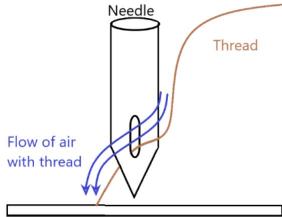
Figure 23 Heat loss by convection due to thread movement
