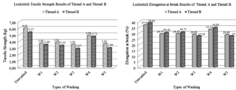
**Figure 5.** Lockstitch tensile strength and elongation at break results of Thread A and Thread B.
