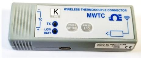
Figure 10 Wireless device for K type
