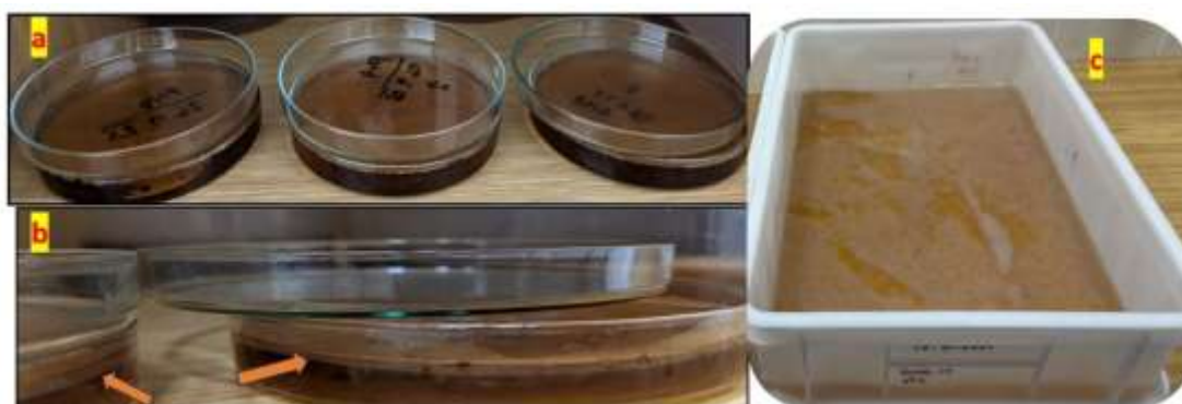
Figure 4.3 Synthesis of BC samples under static cultivation conditions. (a) Growth of BC pellicles in a Petri dish; (b) magnified view of BC pellicles with thickness of approximately 2–3 mm; (c) rectangular plastic container for large-area sample cultivation.
