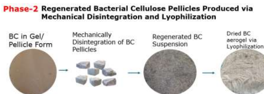
Figure 4.2 Illustration of regenerated bacterial cellulose pellicles produced via mechanical disintegration and lyophilization.
