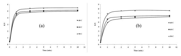
**Figure 19** Effect of drying time and temperature of pad-dry technique on the colour strength (K/S values) of (a) silk fabric and (b) wool fabric dyed with 20 g/l eucalyptus leaf extract and using 20 g/l ferrous sulfate by using simultaneous mordanting
