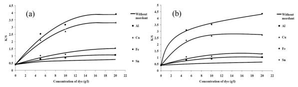
**Figure 11** Effect of dye concentrations on *K/S* values of silk fabric dyed with 10 g/l mordants by pre-mordanting and using (a) pad-batch technique (b) pad-dry technique
