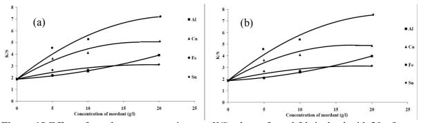
**Figure 18** Effect of mordant concentrations on *K/S* values of wool fabric dyed with 20 g/l eucalyptus leaf extract by simultaneous mordanting and using (a) pad-batch technique (b) pad-dry technique
