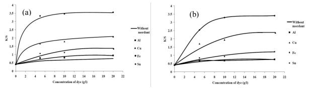
**Figure 13** Effect of dye concentrations on *K/S* values of silk fabric dyed with 10 g/l mordants by post-mordanting and using (a) pad-batch technique (b) pad-dry technique
