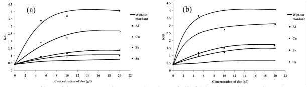
**Figure 12** Effect of dye concentrations on *K/S* values of silk fabric dyed with 10 g/l mordants by simultaneous mordanting and using (a) pad-batch technique (b) pad-dry technique
