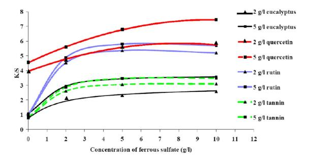
**Figure 21** The *K/S* values of dyed wool fabric with eucalyptus leaf extract, quercetin, rutin and tannin dye by varying concentration of dyes and ferrous sulfate
