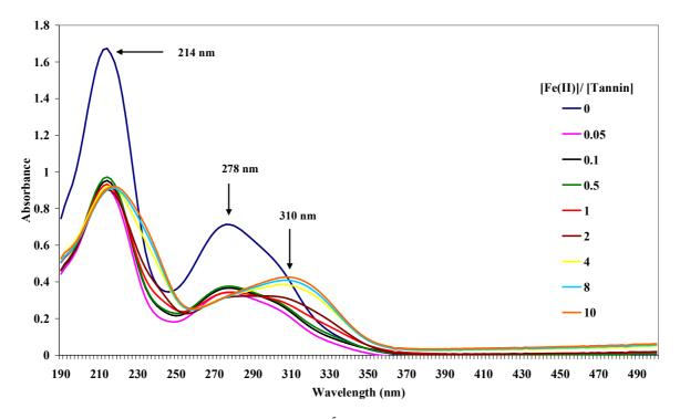
Figure 5 Absorption spectra of tannin  $(1 \times 10^{-5} \text{ Molar})$  in aqueous solution in the absence and in the presence of Fe (II) (0-100 micro molar)
