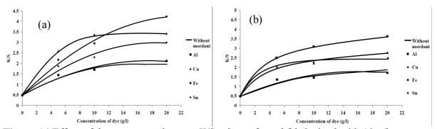
Figure 14 Effect of dye concentrations on K/S values of wool fabric dyed with 10 g/l mordants by pre-mordanting and using (a) pad-batch technique (b) pad-dry technique
