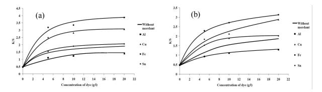
**Figure 16** Effect of dye concentrations on *K/S* values of wool fabric dyed with 10 g/l mordants by post-mordanting and using (a) pad-batch technique (b) pad-dry technique
