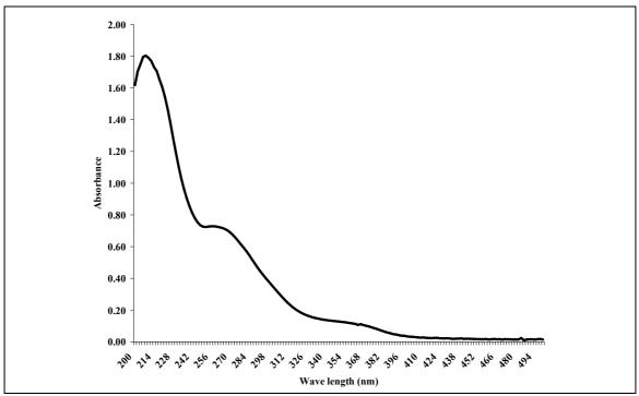
Figure 9 UV-VIS spectrum of 50 mg/l crude eucalyptus leaf extracted dye in distilled water.
