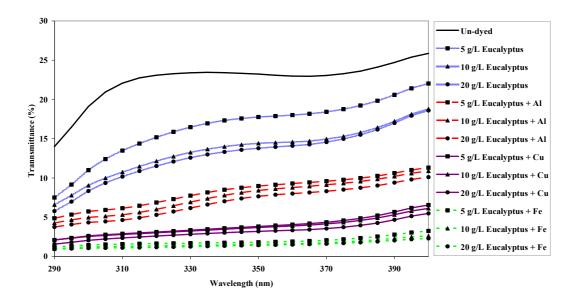
**Figure 23** UV transmission of silk fabrics dyed with eucalyptus leaf extract in the absence and in the presence of metal mordants by the pad-dry technique Note:  $AI = AIK(SO_4)_2$ ,  $Cu = CuSO_4$ ,  $Fe = FeSO_4$
