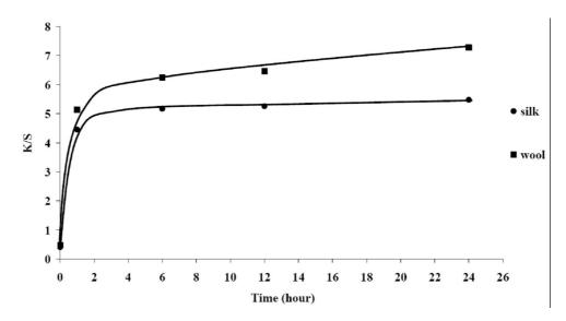
**Figure 20** Effect of batching time of pad-batch technique on the colour strength (*K/S* values) of silk and wool fabric dyed with 20 g/l eucalyptus leaf extract and using 20 g/l ferrous sulfate by using simultaneous mordanting
