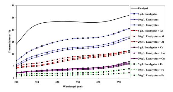
**Figure 24** UV transmission of silk fabrics dyed with eucalyptus leaf extract in the absence and in the presence of metal mordants by the pad-batch technique Note:  $Al = AlK(SO_4)_2$ ,  $Cu = CuSO_4$ ,  $Fe = FeSO_4$
