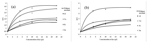
**Figure 15** Effect of dye concentrations on *K/S* values of wool fabric dyed with 10 g/l mordants by simultaneous mordanting and using (a) pad-batch technique (b) pad-dry technique
