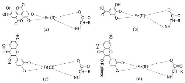
**Figure 22** The proposed structure of Fe (II)/ dyestuff/ wool complexation (a) ellagic acid (b) gallic acid, (c) quercetin and (d) rutin
