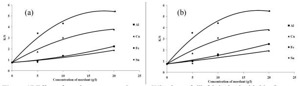
**Figure 17** Effect of mordant concentrations on *K/S* values of silk fabric dyed with 20 g/l eucalyptus leaf extract by simultaneous mordanting and using (a) pad-batch technique (b) pad-dry technique
